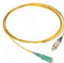
Pigtails with single mode fiber available with SC/APC or FC/PC connector to fusion splice to an incoming fiber
