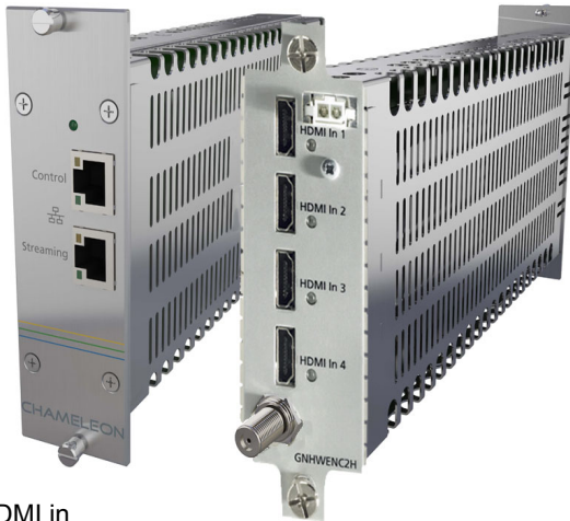
4 x HDMI in MPEG2&4 encoding DVB-T out
